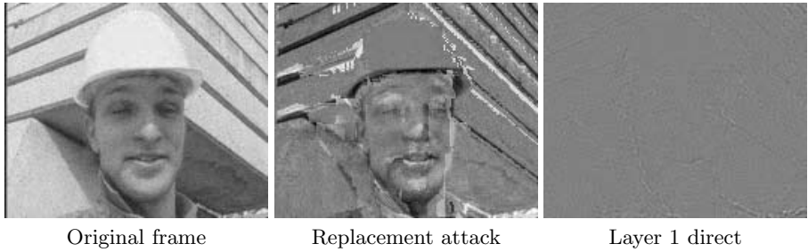
Fig. 5. Reconstructions based on two attacks compared to the original image for the Foreman sequence for the 100th P-frame (GOP with only I-frames)
