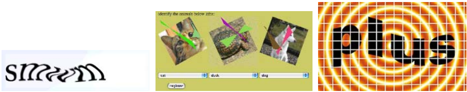
Fig. 1. An example CAPTCHA, which is solved if a user recognizes the word 'smwm' Fig. 2. A sophisticated CAPTCHA, which adds distortion to the image if a user identifies all the three animals Fig. 3. A modern CAPTCHA, which adds a grid pattern to the image
